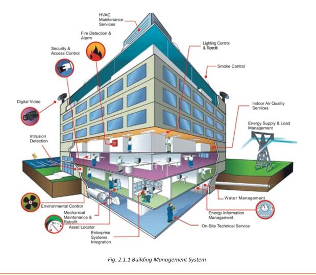
A basic BMS is made up of the relevant software, a server with a database, and smart sensors that are linked to an Internet-capable network. Smart sensors placed throughout the building collect data and transmit it to the BMS, to be recorded in a database. If a sensor sends data outside of pre-defined parameters, the BMS will raise an alarm. In a data centre, for example, when the temperature in a server rack exceeds the permitted limits, the BMS may sound an alarm.
