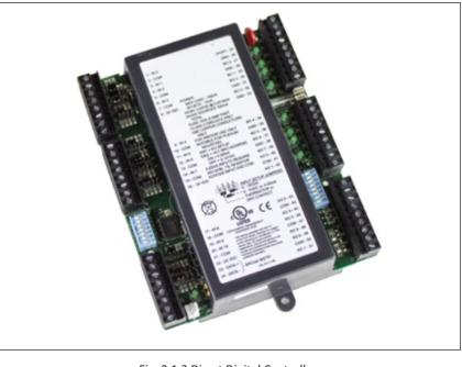
Fig. 2.1.3 Direct Digital Controller
